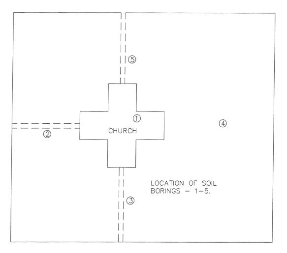
BORINGS #2 & #3 PLACED 30' OFF OF BUILDING. BORING #4 PLACED 50' OFF CHURCH. BORING #5 PLACED 22' OFF BUILDING.
