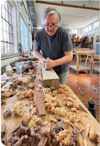
This view captures Kelley Blanton, a cabinet maker who learned his trade in historical joinery in Colonial Williamsburg, planing oak pipes in one of the early stages of construction.
