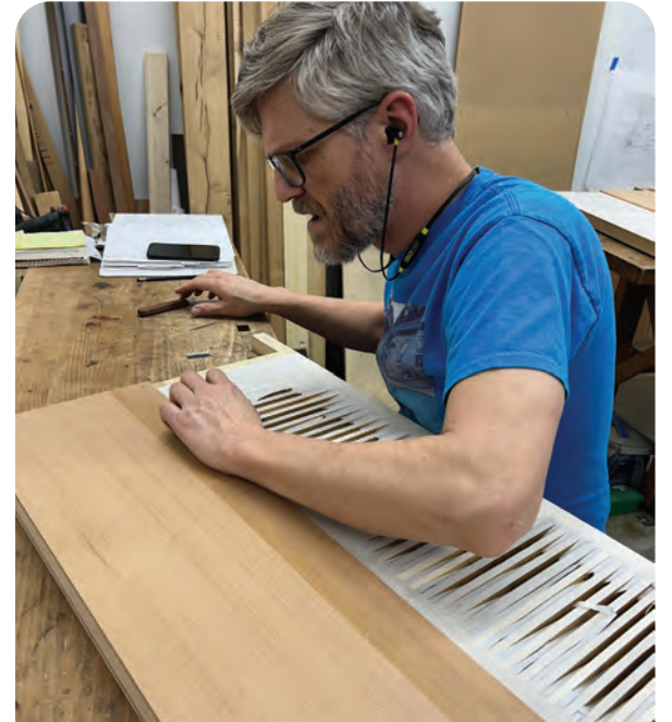
Joel VanderZee, a talented organbuilder and gifted organist from Chicago, cuts open the valve slots under the windchest.
